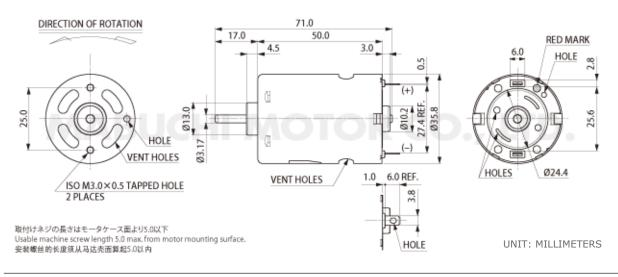
RS-545SH-2860 12.0V 75 75 7,500 5,000 50 5.0 25 2.5 2,500  $b_{2}$ [mN-m] 100 EFFICIENCY [%] CURRENT [A] SPEED [r/min] 500 [g-cm] 1.000 TORQUE
