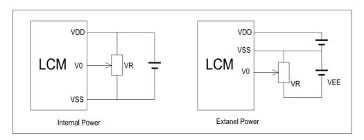
$V_{DD\sim}V_0$ : LCD Driving voltage
