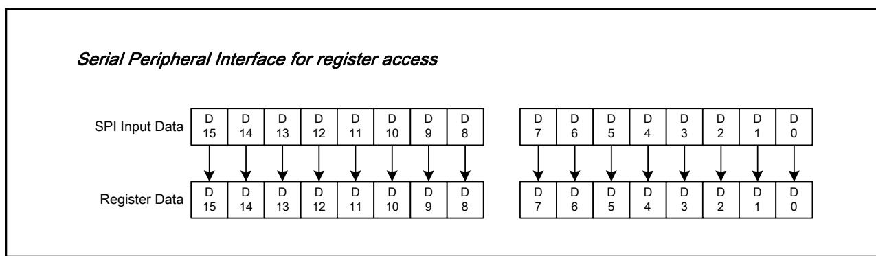
Figure18 Register Setting with Serial Peripheral Interface (SPI)
