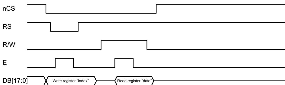
***M68 9-/8-bit System Bus Interface Timing***
