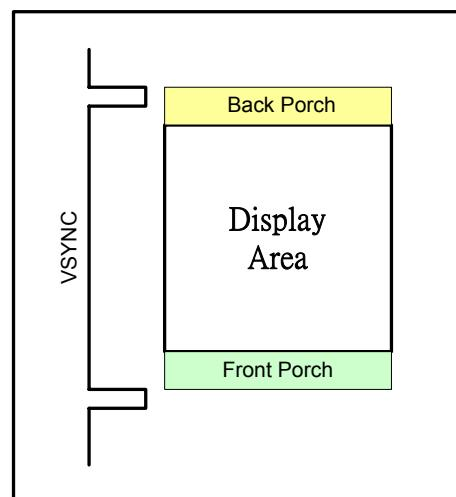
Note: The output timing to the LCD is delayed by 2 lines period from the input of synchronizing signal.
