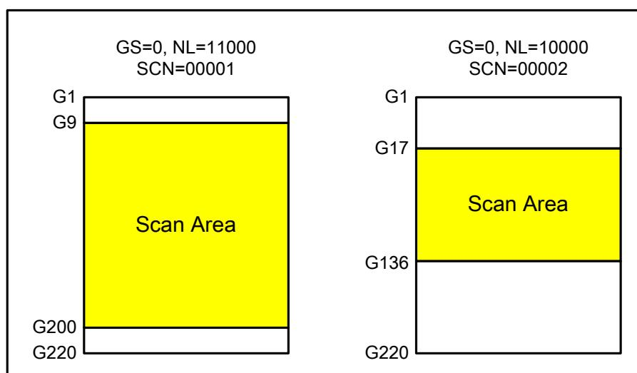
Figure 26 Scanning Start Position for Gate Driver
