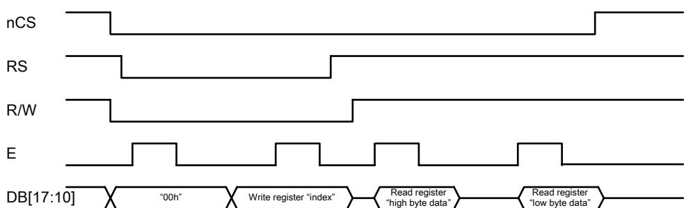
**Figure21 Register Read/Write Timing of M68 System Interface**
