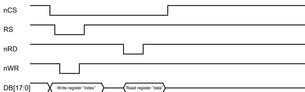
***i80 9-/8-bit System Bus Interface Timing***
