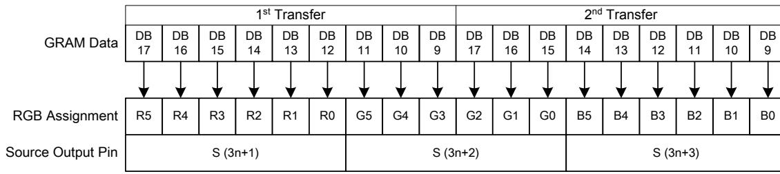
GRAM Data and display data of 18-/9-bit system interface (SS="0", BGR="0")
