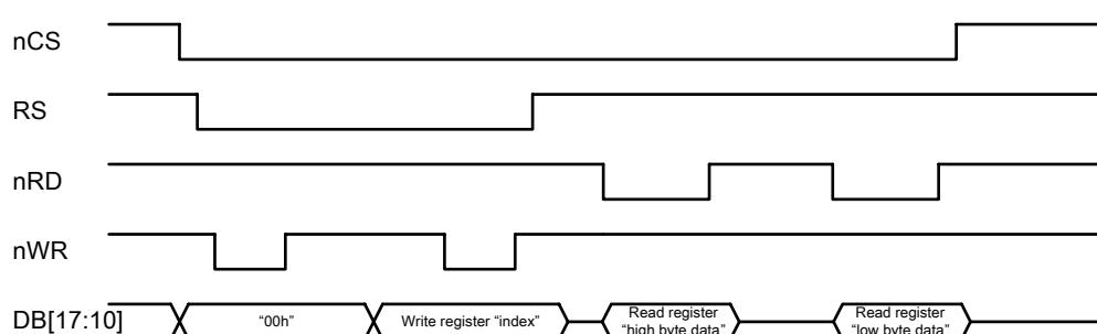
**Figure20 Register Read/Write Timing of i80 System Interface**
