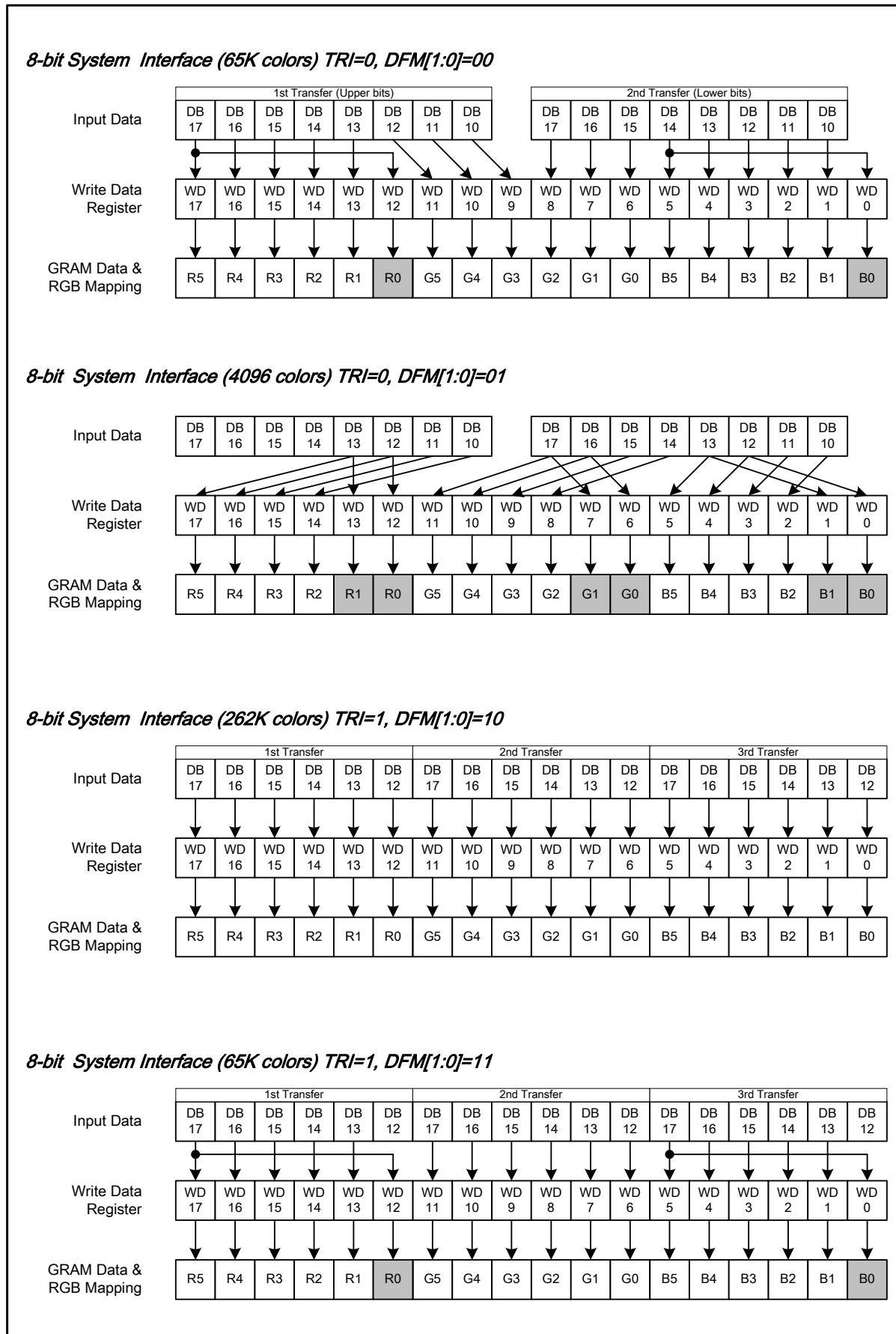
**Figure5 8-bit System Interface Data Format**
