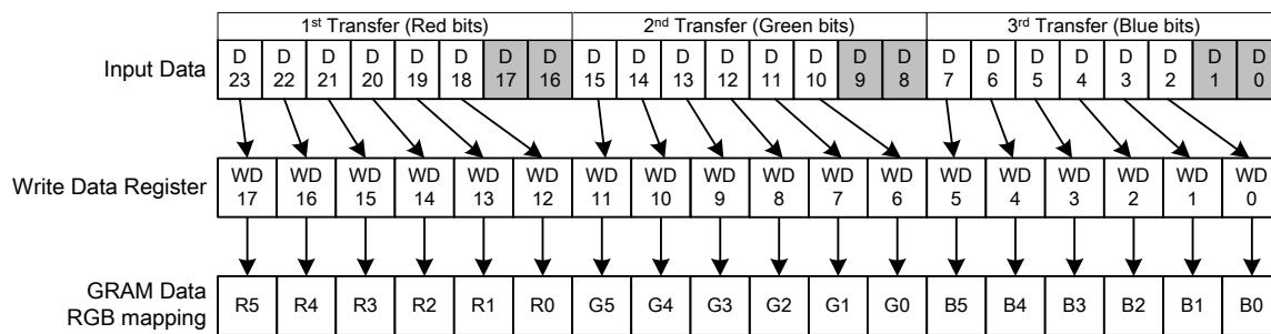
**Figure7 Data Format of SPI Interface**
