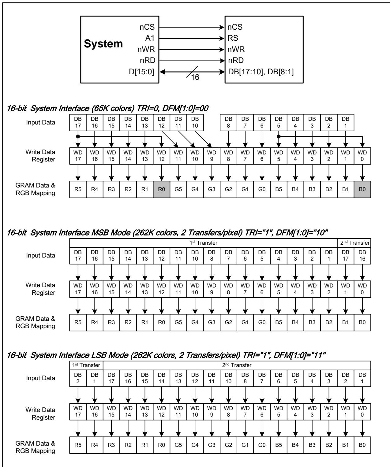
Figure3 16-bit System Interface Data Format
