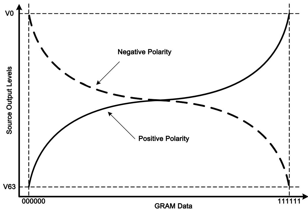
Figure38 Relationship between GRAM Data and Output Level
