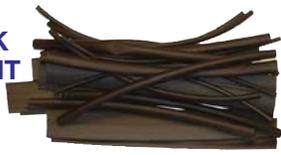
24 pc. of 6in. long Black Shrink tubing in assorted Dia. Flexible polyolefin rated for 125 deg. "C"/600V. Listed dia. before shrinking. 4 pcs. each of following sizes: 3/32", 1/8", 3/16", 1/4", 3/8" & 1/2"
