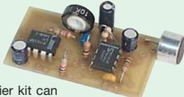
Super sensitive amplifier kit can hear through walls etc. Couple to a parabolic reflector & earphones to hear for blocks. Based on the LM386 ChipCan be used as a general purpose 1.5W amp. Supplied with a mini-microphone. Runs on 6-12V DC. AA-1D
