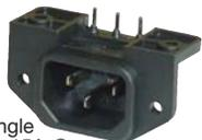
IEC 60320 type C-14 Right Angle P.C. mount, power inlet. Rated: 15A @ 250VAC UL/CSA. Standard IEC equipment end male 3 blade cord connector. Solder terminals.
