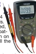
Talking, back lit, auto ranging, 3-3/4 digit, multimeter with Lighted test leads. Rubber case for protection. Soft sided, zippered belt case. Requires 3 "AA" batteries (not included). Pressing button on Red Test Probe causes meter to tell the Range & Value
