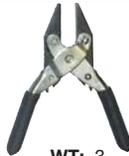
AKA "Fishermans" pliers. 5" long with hardened parallel opening smooth jaws. Cushioned grips. 7/16" max. opening X 1-1/8" depth.
