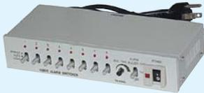
Rugged metal cabinet. Lighted power switch, LED source Indicator. 3 sequencing modes; Auto, Manual, Home. 3 alarm modes: ON: Internal buzzer sounds, video switches to associated input, Alarm relay activates; BUZZER OFF: No buzzer sound, video switches to associated input, alarm relay activates; OFF: no alarm functions. Alarm overrides all sequence modes CE Listed
