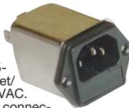
POWER DYNAMICS HGN-365-6M-F1, Flange mount, power inlet/ RFI Filter. Rated: 6A @ 125/250VAC. Standard male 3 blade IEC cord connector and fuse holder. .250 quick connect output terminals, 5 X 20mm type fuse. UL/CSA listed.
