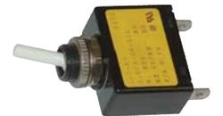
AIRPAX B11-2-2.00A-06-11L, circuit breaker/switch rated: 250VAC, 50/60 Hz; 50VDC; Carry 2A Trip 2.7A. Magnetic type with 5/8" white handle. Mounts in 1/2" "D" hole. .250" Quick connect terminals. UL/CSA listed.
