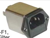
POWER DYNAMICS HGN-365-6M-F1, Flange mount, power inlet/RFI Filter. Rated: 6A @ 125/250VAC. Standard male 3 blade IEC cord connector and fuse holder. .250 quick connect output terminals, 5 X 20mm type fuse. UL/CSA listed.
