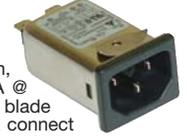
DELTA 06DENG3B-R, Snap-in, power inlet/RFI Filter. Rated: 6A @ 125/250VAC. Standard male 3 blade IEC cord connector. .250 quick connect output terminals, UL/CSA /VDE listed.
