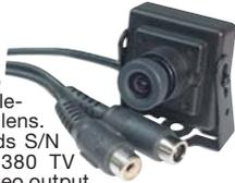
Ideal for use with Telephoto Lens 12975-LN. 1/3" CCD element with Fixed 3.6mm lens. Scanning 525 lines-60 fields S/N ratio:>46dB, Resolution: 380 TV lines, Sensitivity: .1 lux, Video output : EIA 75 Ohm, 2/1 interlace 1.0V P/P composite video. Metal housing with removable mounting bracket. Auto iris/shutter: 1/60/-1/100,000 sec. Connections: 6ft cable, Video/ RCA Female, Power/ Coaxial. Power 12VDC +/-5V @ 120mA. Sq: 1" W/O bracket" D: 1-3/16" WT: .24
