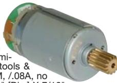
Johnson 24 VDC motor with Bronze sleeve bearings. Similar to HC685LG. Used in tools & appliances etc. 4600+RPM, .708A, no load, 3A Stall @ 24V. 1/8" [Dia.] X 7/16" steel front shaft with 1/2" Dia. 14Tooth Brass gear, 1/8" Dia. X 5/16" rear shaft. Rear mounted removable circuit board with 4 Pin mini header and a PTC resettable fuse (1.3A hold). Two m3.3 tapped mounting holes in front.
