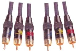
Premium Stereo audio & composite video cable made with Oxygen free copper wire. Left & Right Stereo cables & video coax. Copper braid & aluminum foil double shielding. 24kt gold plated Red, White & Yellow coded RCA Plugs with metal shells.
