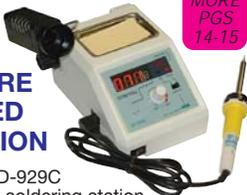
ZD Electronic Tools ZD-929C Temperature controlled soldering station with LED display. Heat sensor located near the tip for fast response and +/-10° "F" control. Rated at 48Watts, 24VAC handle. Temperature range: 320° "F" to 800° "F". Isolated tip, fused line. 117 VAC. Extra tips are available for general replacement or special uses.
