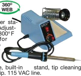
General purpose solder station for the hobbyist. Adjustable from 5 to 50 Watt (800° F max) heat output for repairing PC boards to soldering transformer terminals. Station provides on-off switch, knob to control wattage, built-in stand, tip cleaning sponge & 1/32" point tip. 115 VAC line.
