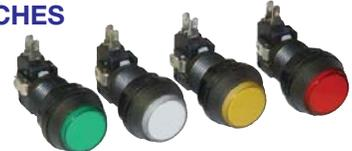
Lighted, large plastic body, panel mount SPDT push button switches. Mount in a 15/16" hole. 1/4" quick connect terminals. Switch Contacts: 5A @ 250 VAC. Replaceable wedge base Lamp: rated 12V @ 3W, L: 2-1/2" WT: .065
