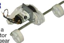
USED Motor assembly with a Buehler 1.16.025.031.00 motor driving a 6 piece plastic gear train. Center driven, 6-7/8" long output shaft drives two 1-5/16" Dia. off center plastic cams attached near ends. Approx. 116 RPM @ 12VDC. 5-1/4" C/C distance on cams. We guess that it was part of a paper feed.
