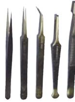
5 piece assortment of stainless steel tweezers in a plastic hanging pouch. Includes: needle, spade, bent, blunt & flat.
