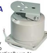
Motorized scanner unit for security cameras. Supports cameras up to 2kgs. Scans back and forth automatically up to 350deg's. Externally adjustable limit stops. Manually adjustable tilt(90deg.) . 24VAC power. 6in leads. Off white plastic case, metal camera mount. Indoor use only.
