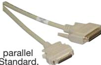
IEEE 1284 compliant, 10ft. parallel printer cable. For use with Standard, ECP & EPP printer ports. Cable has a DB-25 male on one end and a 36pin Half Pitch Centronics male on the other. Platinum jacket with with foil & braided shielding. Molded strain relief on connectors.
