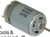
Johnson 13.6VDC motor with Bronze sleeve bearings. Used in tools & appliances etc. 6100+RPM, .44A, no load, @ 13.6V. Max Torque: 6.1oz/in @ 13.6V/2.8A 1/8" [Dia.] X 3/4" serrated steel shaft. Solder terminals. 2 mounting holes threaded M3 on front.
