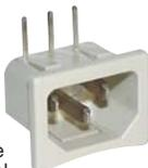
PC mount, white thermoplastic, 220 VAC @10A IEC 60320 type C-14 three wire primary power connector. 3 PC solder pins plus 1 ground solder lug for chassis connection. UL/CSA & major world agencies approved.
