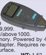
Hand held photoreflexive tachometer uses LASER beam. 5 digit LCD display measures RPM from 2.5-99,999. Resolution: .1RPM/2.5-999, 1RPM/above 1000. Features Hi/Lo/ Last reading memory. Powered by 4 "AA" cells or included 120VAC adapter. Requires reflective area on a non reflective surface.
