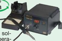
40W Temperature controlled soldering station with digital temperature control & display, grounded tip, ceramic heater and comfort grip handle. Easy off connector for easy replacement of handle/heater. Adjustable Temperature range: 200 deg. "C" to 480 deg. "C" (392-896 "F"). Fused line. 117 VAC. WT: 4.7
