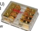
Distribution block for Type AUE (AGU) fuses. All metal parts are 24K Gold plated. Holds 4 AUE (AGU) fuses up to 80A each. One 3 way #4 AWG input, Four 8AWG output. Inner steps to allow insulation into block. Set screw clamps, clear housing.
