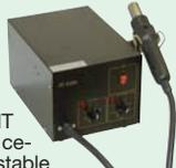
Hot air repair/rework station for SMT devices. Features: a fast heating ceramic heater, internal air supply, stable temperature, comfort grip handle, interchangeable hot air nozzles for PLCC/SOP/ etc. devices. Adjustable temperature & air flow. Temperature range: 150 deg.-500deg. "C".
