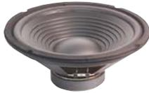
8ohm Impedance, 10" poly-propylene woofer rated: 20oz magnet, Frequency Range: 28Hz-4KHz, 100 peak power, SPL= 89db, resonant freq. =30Hz.
