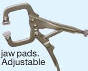
"Welding" style clamping pliers. Drop forged jaws. 1-1/2" Throat depth, 1" Jaw capacity, 1/2" dia. jaw pads. For welding, soldering or gluing. Adjustable locking grip with release.
