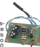
Circuit output is open collector transistor that sinks up to 80mA to operate external relay (NOT SUPPLIED). Holds relay closed until temperature rises to adjustable set point. Range Approx. -20 to +300°F. 7.5-15V DC Operation. TG-2D
