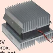
Peltier Effect cooling assembly. Contains module with 127 Pairs of couples mounted to a heatsink assembly. Optimized for 12VDC. 65-70W (~170 BTU). 8A max, 16V max, Draws 6A @ 12VDC. Approx. 50Deg "C" temp. difference with hot side fan (Not included) and insulated cold side. Designed for recreational coolers.
