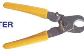
8" Heavy duty cutter for cutting soft copper wire up to 2/0 or communication cable up to 100 pairs. Not for hard drawn copper wire, steel core or steel supported coax cable.
