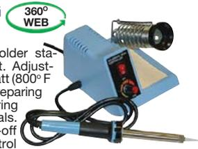
General purpose solder station for the hobbyist. Adjustable from 5 to 50 Watt (800° F max) heat output for repairing PC boards to soldering transformer terminals. Station provides on-off switch, knob to control wattage, built-in stand, tip cleaning sponge & 1/32" point tip. 115 VAC line.
