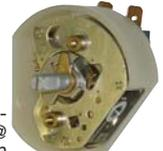
Robertshaw 10min. timer. SPST contacts rated 20A Resistive, 1/3hp @ 120/240VAC. Contacts close when you turn the shaft, times out from what you set. (Min. approx. 1min). 1/4" Dia. double flat, split shaft 11/16" long. Back of panel mounts with two 4-40threaded inserts. .250" quick connect terminals.
