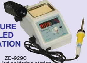
ZD Electronic Tools ZD-929C Temperature controlled soldering station with LED display. Heat sensor located near the tip for fast response and +-10° "F" control. Rated at 48Watts, 24Vac handle. Temperature range: 320° "F" to 800° "F". Isolated tip, fused line. 117 VAC. Extra tips are available for general replacement or special uses. Base L: 6-3/4" X W: 4-3/4" X T: 3-9/16" WT: 4.8
