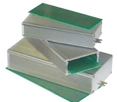
Extruded aluminum case with mounting flanges on end plates. Natural Aluminum finish on case and end plates. Slots for PC Board on inside. Grooved outside with smooth end plates. Includes Double Sided FR-4 board with Plated Through .032 holes on .1" spacing. Board For 17804 BX contains 20X57 Holes Board For 17805 BX contains 24X67 Holes Board For 17806 BX contains 32X77 Holes I/D listed below
