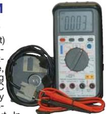
Quality 3-3/4 digit (3999 count) DMM with 1" char. ht. Connects to your PC port & software provides data capture, tracking & printing. Autoranging or manual, Data Hold, AC & DC voltage/Current, frequency to 30KHz, Capacitance, Resistance, 40M Ohm, Fused input. Includes Test leads, Black Boot, RS232 cable & Software. Requires: Pent. 90MHz or better, Win95 above, 16M RAM, 20M Hard drive space, Floppy Drive. **Batteries not included**
