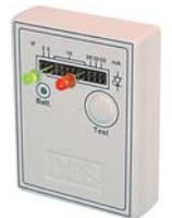
Compact, pocket sized checker/comparator for LEDs. 12 position test socket strip provides tes currents of 2,5,10,20,30 & 50mA. 7 center positions provide 10mA test current allowing you to compare several LED at the same time. Requires 9V battery (not supplied)
