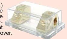
Heavy duty Type ANE (ANL) fuse block. All metal parts are 24K Gold plated. Holds single ANE/ANL fuse up to 500A. Accepts up to 1AWG cable, Set screw clamp, clear snap on cover.
