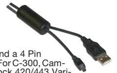
KODAK, USB cable with a Type A male on one end and a 4 Pin Mitsumi Male on the other. For C-300, Camera Dock 6000, Dock II, Dock 420/443, Various CX, DX, LX cameras, Printer Dock, Dock 4000,6000, Plus. Black jacket with molded black strain relief on connectors. Ferrite filter on Mini Mitsumi end
