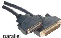
IEEE 1284II compliant, 15ft. parallel printer cable. For use with Standard, ECP & EPP printer ports. Cable has a DB-25 male on one end and a Half Pitch Centronics male on the other. Black jacket with foil & braided shielding.
