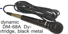
600 ohm unidirectional dynamic microphone features: DM-68A Dynamic (moving coil) cartridge, black metal wind screen & body, On/Off switch, 15ft. low noise cable. Sensitivity: -74db, Frequency response: 80-12KHz. Cable has XLR female mike connector on one end & a 1/4" phone plug on other end. Includes a storage pouch & 1/4" to 1/8" phone adapter
