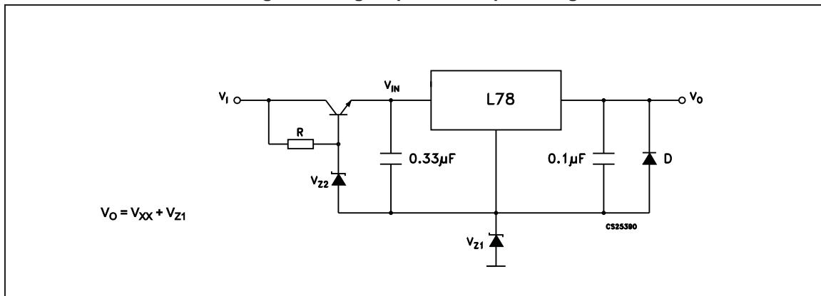
Figure 22. Reducing power dissipation with dropping resistor
