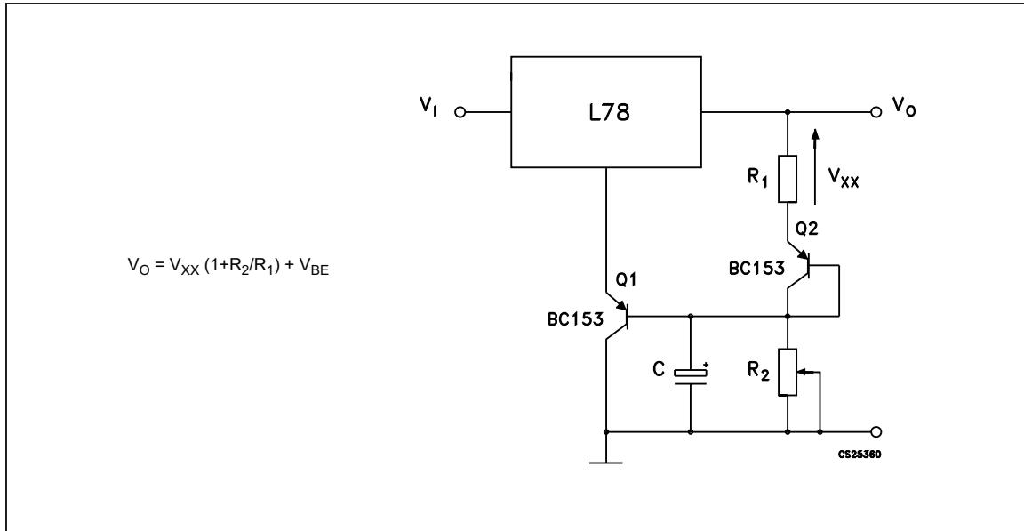
Note:  $Q_2$  is connected as a diode in order to compensate the variation of the  $Q_1 V_{BE}$  with the temperature.  $C$  allows a slow rise time of the  $V_O$ .
