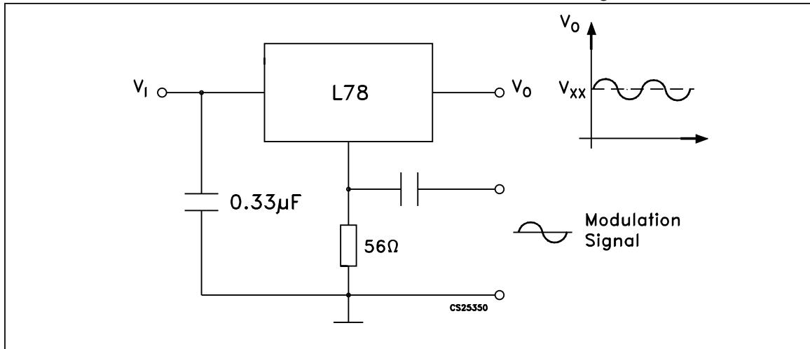
Note: The circuit performs well up to 100 kHz.
