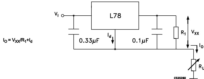
Figure 10. Circuit for increasing output voltage
