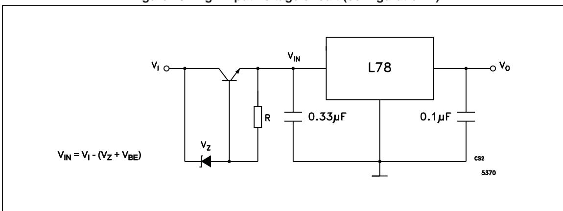
Figure 20. High input voltage circuit (configuration 2)
