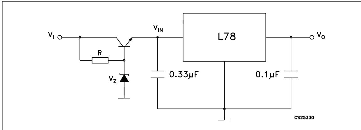
Figure 21. High input and output voltage
