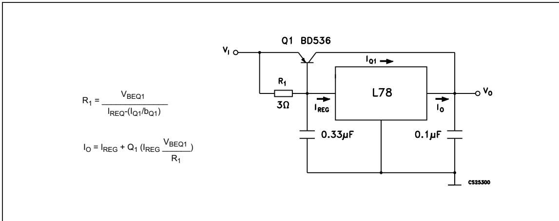
Figure 14. High output current with short circuit protection
