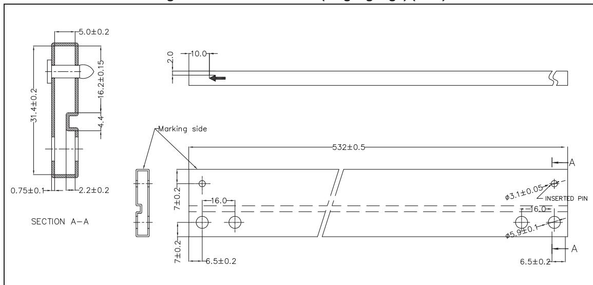
Figure 47. Tape for DPAK and D<sup>2</sup>PAK
