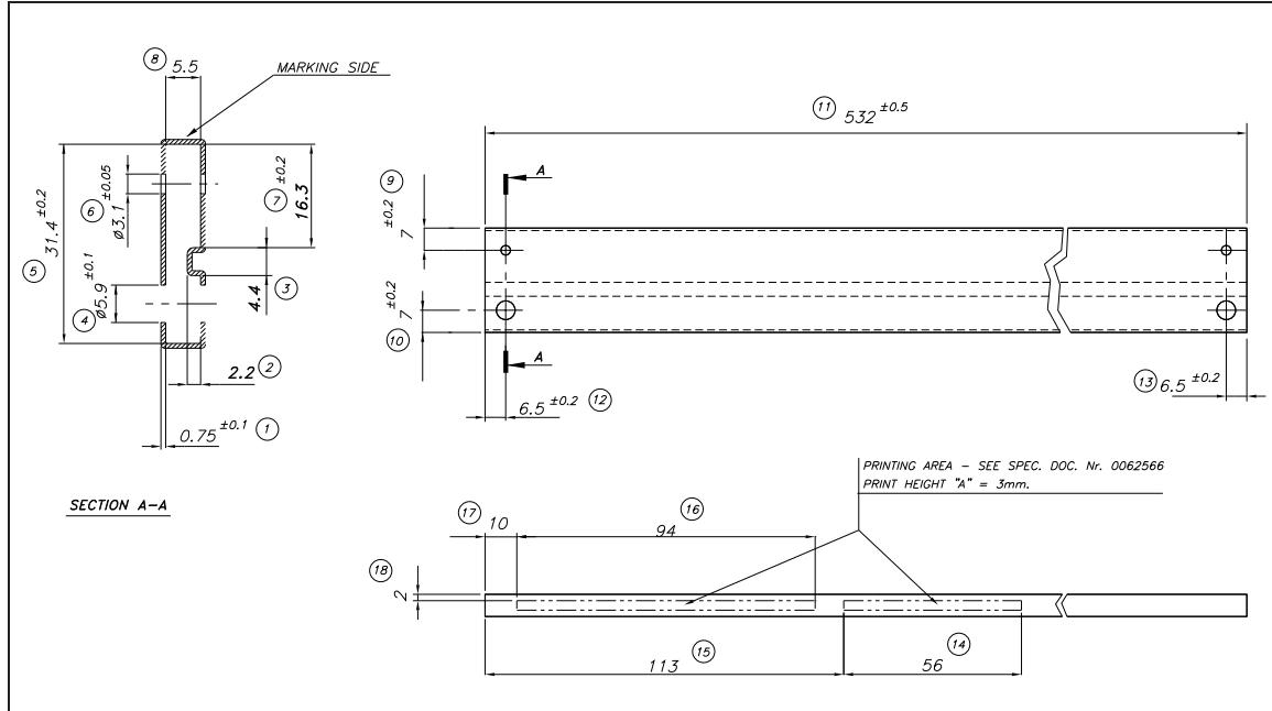
Figure 46. Tube for TO-220 (single gauge) (mm.)
