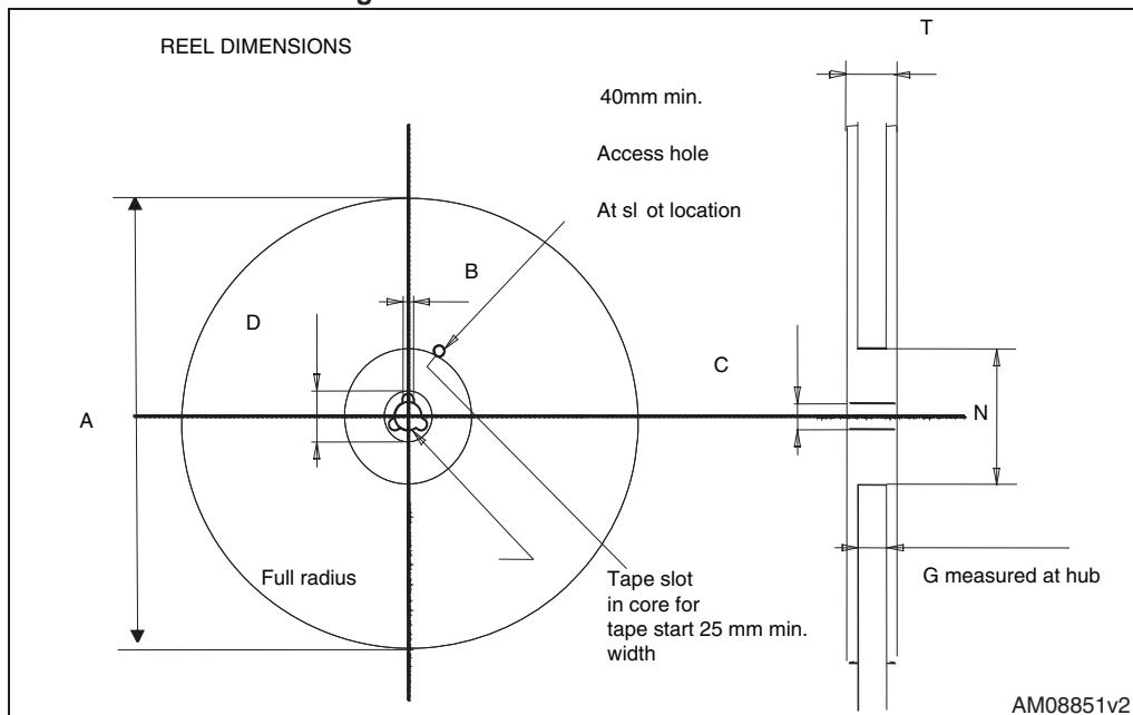
**Table 25. DPAK and D<sup>2</sup>PAK tape and reel mechanical data**
