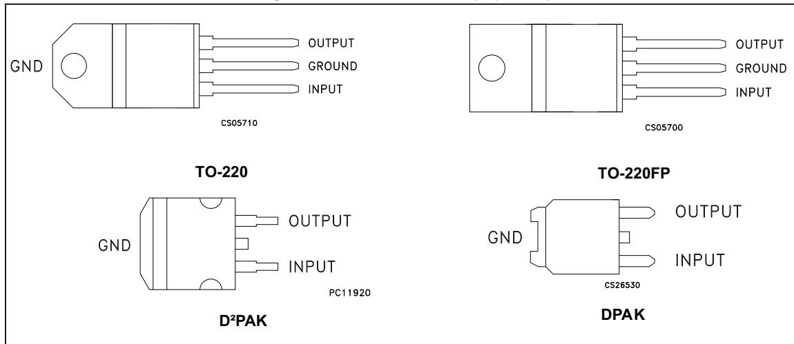
Figure 3. Schematic diagram
