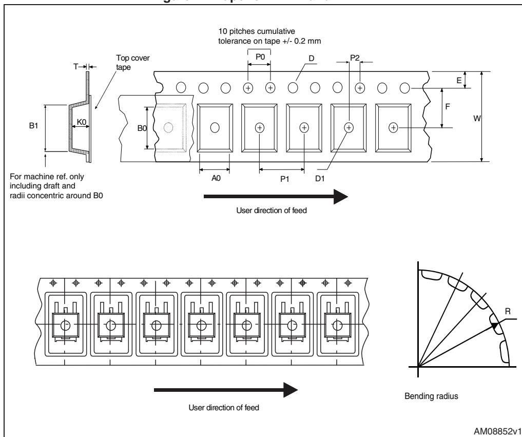
Figure 48. Reel for DPAK and D<sup>2</sup>PAK
