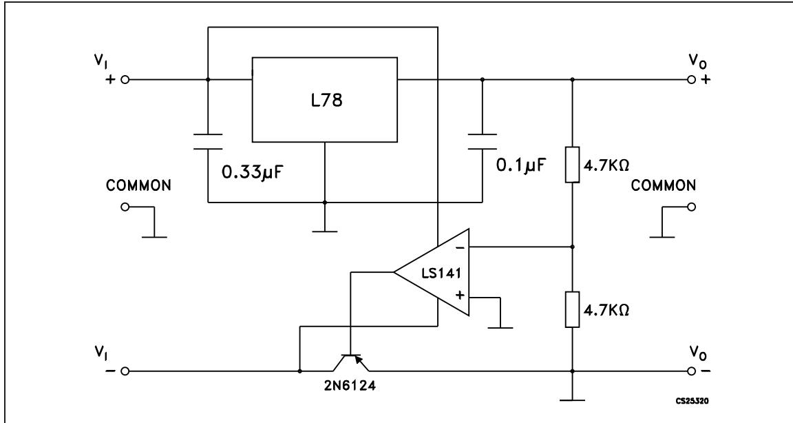
Figure 16. Split power supply ( $\pm 15$  V - 1 A)
