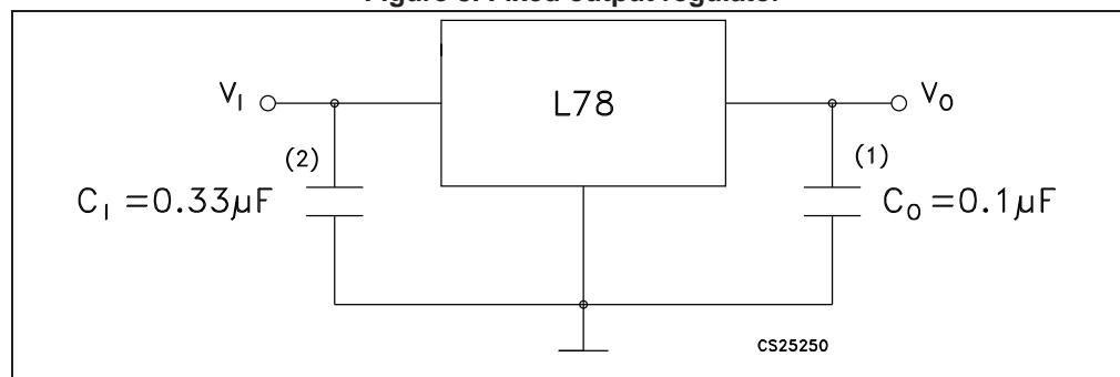
1. Although no output capacitor is needed for stability, it does improve transient response.
