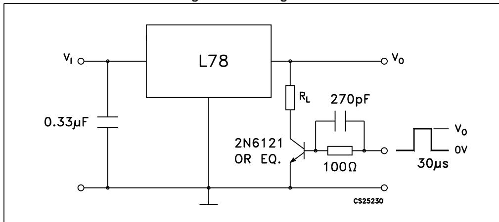
Figure 7. Ripple rejection
