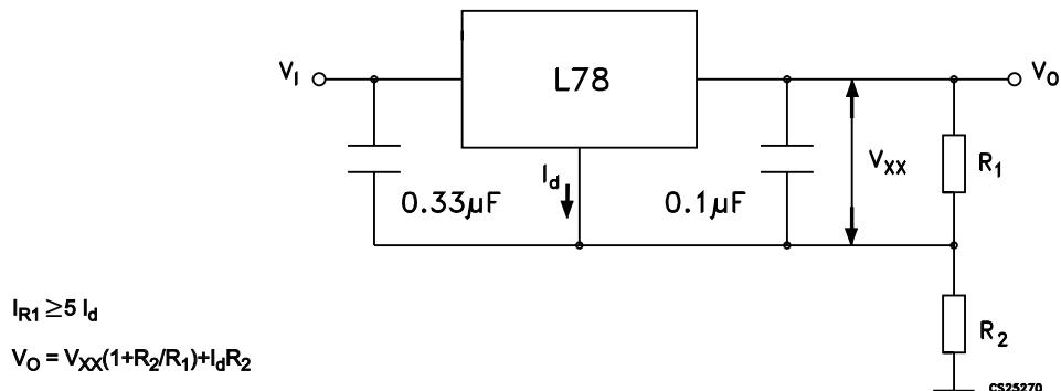
Figure 11. Adjustable output regulator (7 to 30 V)
