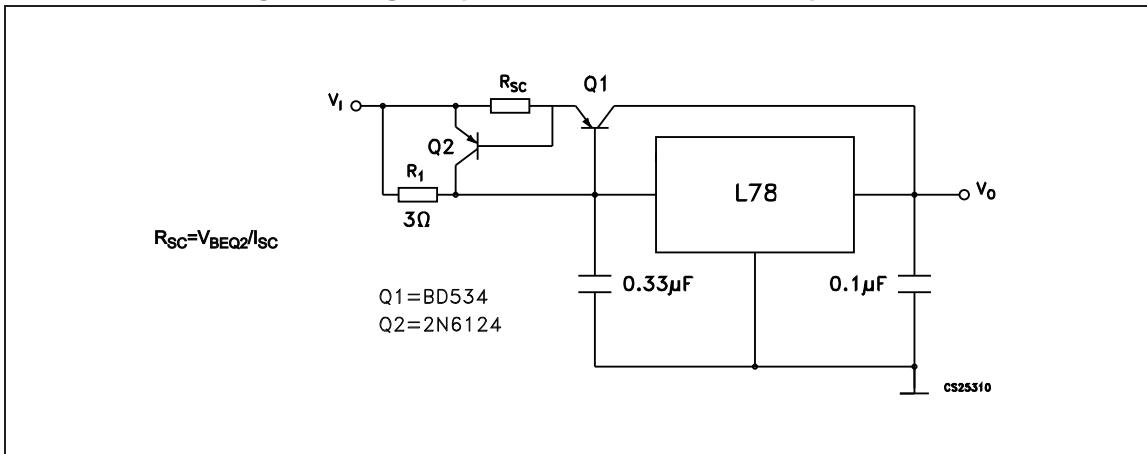
Figure 15. Tracking voltage regulator
