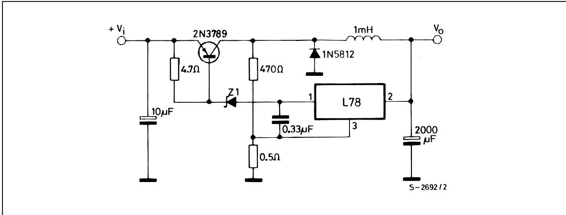
Figure 19. High input voltage circuit (configuration 1)
