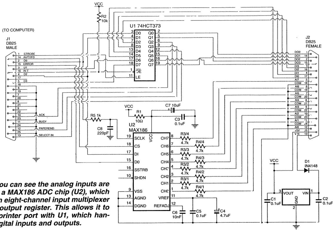
**Fig.1:** As you can see the analog inputs are provide by a MAX186 ADC chip (U2), which includes an eight-channel input multiplexer and serial output register. This allows it to share the printer port with U1, which handles the digital inputs and outputs.
