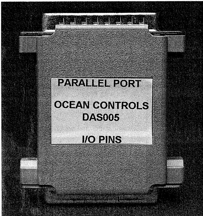
*The author's prototype for the DAQ module, shown here a little larger than actual size. It's built inside a DB-25 'gender bender' backshell, yet provides no less than eight analog inputs, four digital inputs and four digital outputs.*
