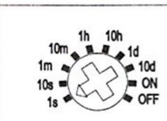
Knob 1: delay gear setting, "s" for second, "m" for minute, "h" for hour, "d" for day, "ON" for relay action (15-18/25-28 closed), "OFF" for relay open (15-18/25-28 open).
