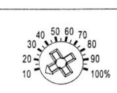
Knob 2: fine adjustment of delay time, 10% ~ 100% adjustable.
