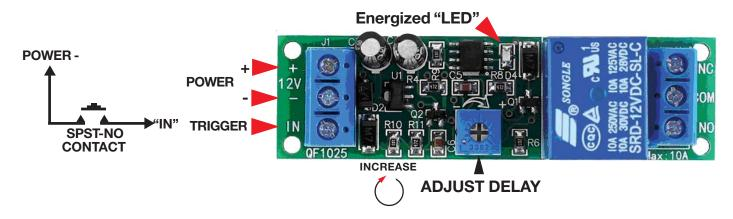
Adjustable General use relay module provides approximately 1sec -60sec. Delay on OFF (Break). Trigger Input turns Relay ON & starts Turn OFF delay Time, after delay, Relay turns OFF **NOTE:** Trigger is locked out for entire timing cycle.
