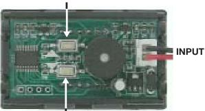
Setting the Upper & Lower Voltage Alarm Limits
