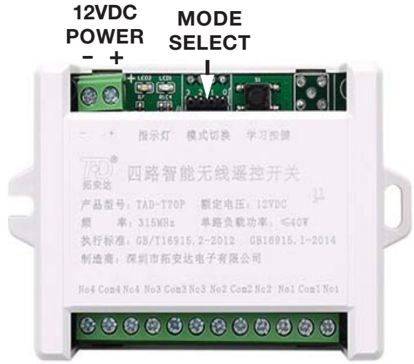
RELAY TERMINAL STRIP
