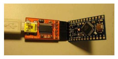
The Arduino Pro Mini connected to (and powered by) a SparkFun FTDI Basic Breakout Board and USB Mini-B cable. Note that on earlier Pro Mini boards the orientation of the 6-pin header may be reversed; check that the words GRN and BLK align on the Pro Mini and FTDI Basic Breakout.
