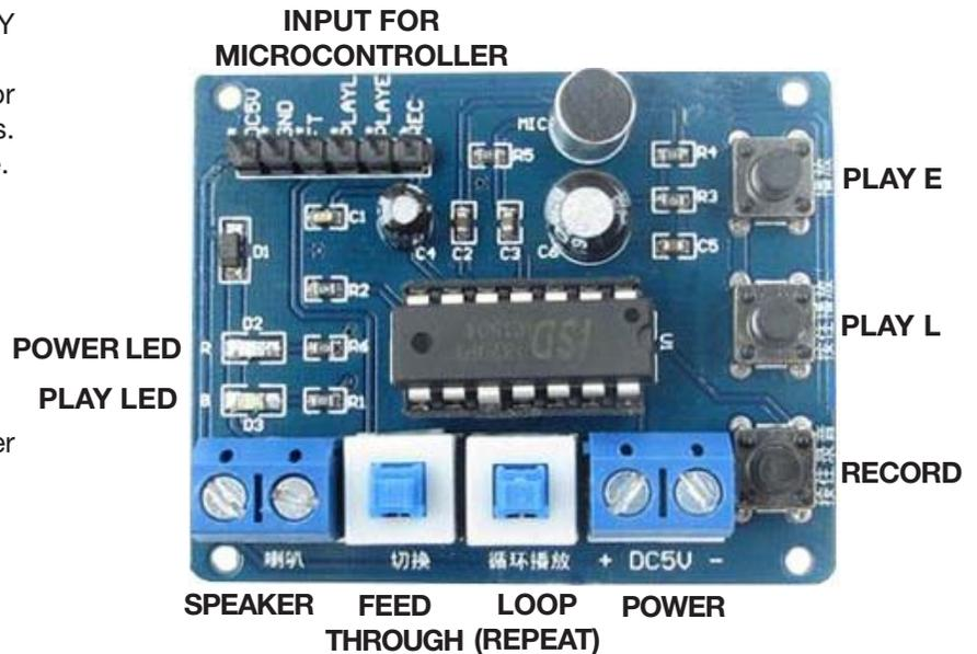
**FEED THROUGH & LOOP SWITCHES ARE ALTERNATE ACTION (PUSH-ON/PUSH OFF)**
