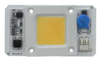
NOTE: AC Line Connections are Spring Loaded, Grip, Push-In.
