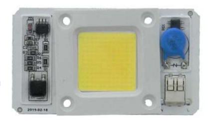
NOTE: AC Line Connections are Spring Loaded, Grip, Push-In.
