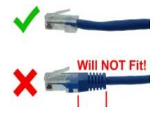
NOTE: FOR RJ-45 PLUGS WITHOUT STRAIN RELIEF
