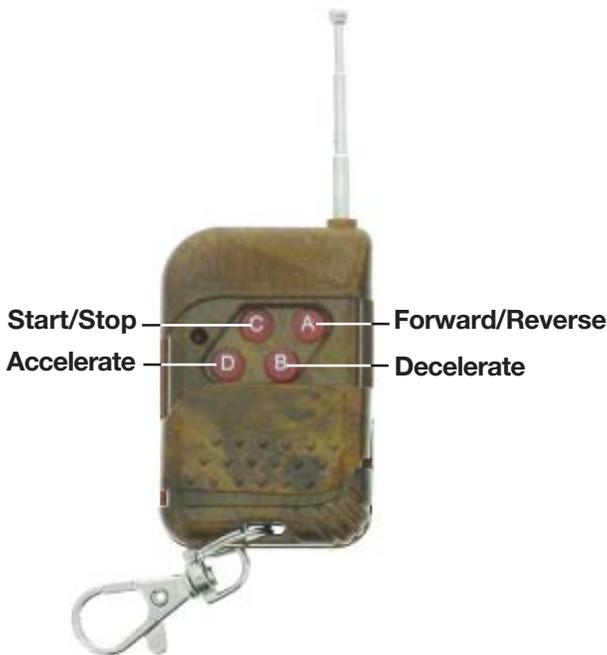
Factory default is both FOB (Transmitter) and the Receiver Address Bits are Floating, So all receivers will respond to all FOBs. This can be changed BUT since the Receiver is soldered to the Motor Driver Board this is difficult AND will void any warranty
