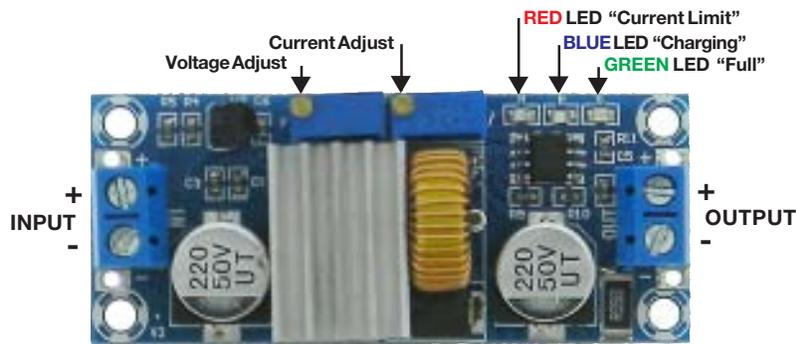
**NOTE: Depending on Input to Output Voltage difference & Load Current Heatsink will get Hot**
