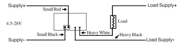
Separate Meter Power 4.5-28VDC
