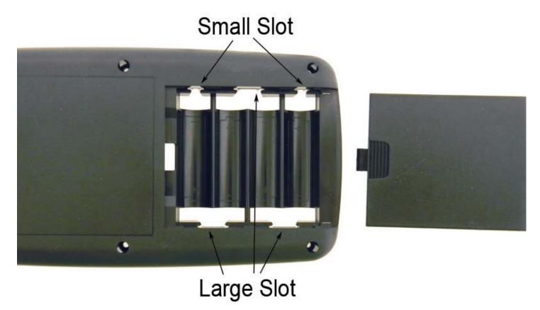
Slide open the battery compartment cover. Working from the outside of the box, locate two small tab slots and three large tab slots. Slide the appropriate tab until locks in position.
