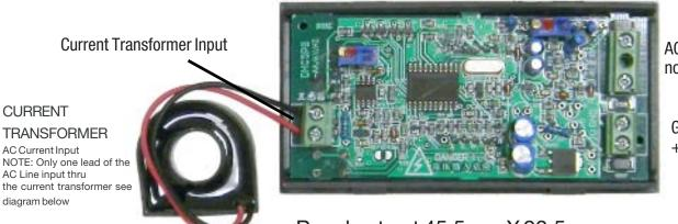
AC Voltage input not polarity sensitive
