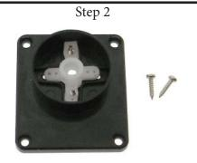
Use screws to mount horn to base (A).
