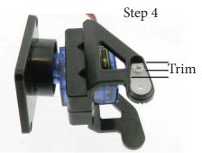
Trim plastic horn from servo with a knife (carefully) to fit in (C) and insert screw.
