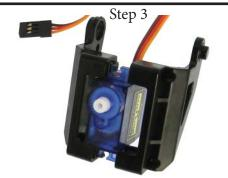
Slide parts (B) and (C) over mounting tabs of a servo, do not use screws at this time, you will need wiggle room later.
