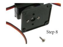
Insert screw though bottom to tighten servo to base.
