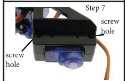
Insert screws to tighten (B) and (C)
