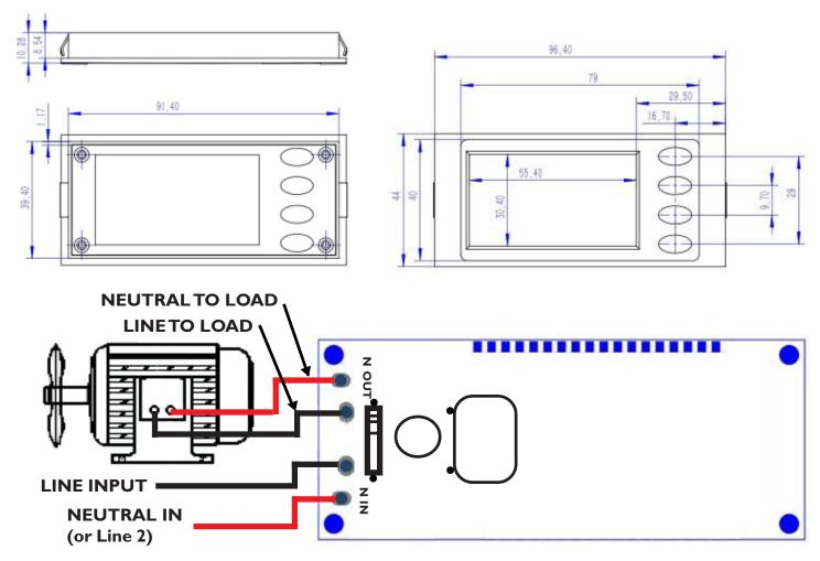
For 120VAC Single Phase: Connect Line to Red Line Lead, and Neutral to Black "N IN" Lead For 220VAC Single Phase: Connect Line 1 to Red Lead, and Line 2 to Black "N IN" Lead
