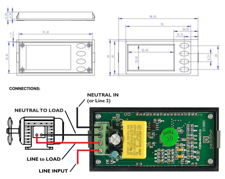
For 120VAC Single Phase: Connect Line to "Line Input" Terminal, and Neutral to "Neutral In" Terminal For 220VAC Single Phase: Connect Line 1 to "Line Input" Terminal, and Line 2 to "Neutral In" Terminal
