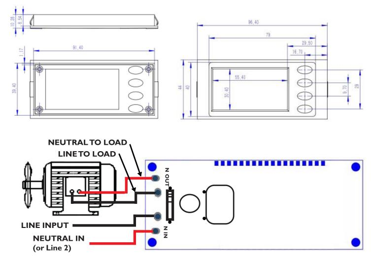
For 120VAC Single Phase: Connect Line to Red Line Lead, and Neutral to Black "N IN" Lead For 220VAC Single Phase: Connect Line 1 to Red Lead, and Line 2 to Black "N IN" Lead
