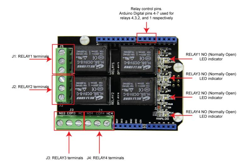
Relay Shield V2.0 terminal connections description
