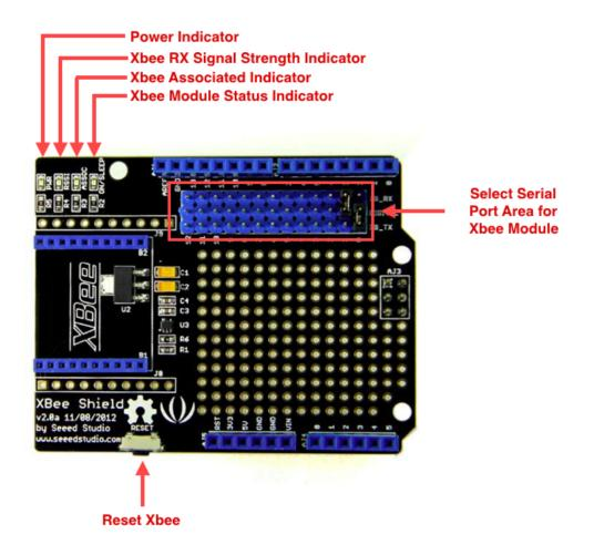
Use a jumper cap to connect XB\_TX and Digital 4. Also, Use a jumper cap to connect XB\_RX and Digital 5. Of course you can change the digital port as you like. But don't forget to change the port number in the definition of the demo code at the same time.
