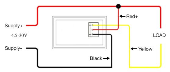
NOTE: Supply lead to & Return Lead from Load to Meter (Yellow) and Meter Common (Black) to Supply should be sized to carry maximum expected Current
