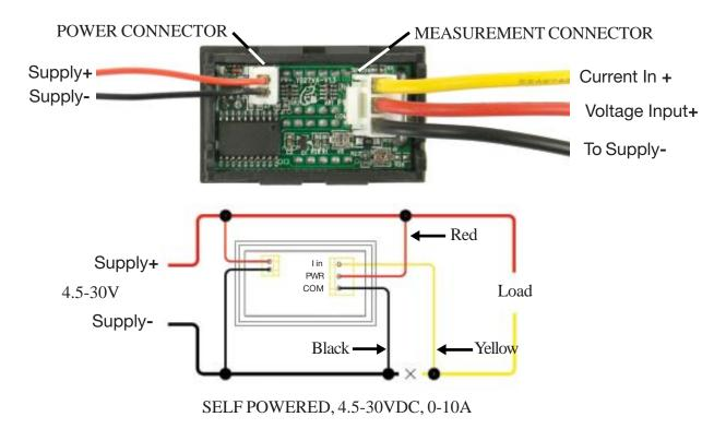
Supply lead to & Return Lead from Load to Meter (Yellow) and Meter Com to Supply should be NOTE: sized to carry maximun expected Current
