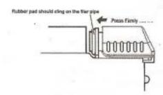
B: The nozzle is damageable. Therefore, it should be cleaned if the solder is not being absorbed.
