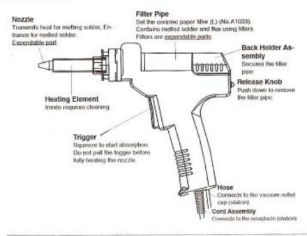
WARINING: Since the desoldering gun can reach a very high temperature, please work carefully. Except when cleaning the nozzle and heating element, always turn the power switch off and disconnect the power plug before performing any maintenance procedure.
