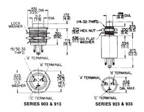
903, 913 SERIES, FRONT MOUNT, .469 MOUNTING HOLE 923, 933 SERIES, FRONT MOUNT, .250 MOUNTING HOLE
