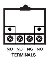
Each switch module contains a SPST-NO and a SPST-NC. To Configure as a SPDT switch you must jumper a NC terminal to a NO terminal to create a "Common"
