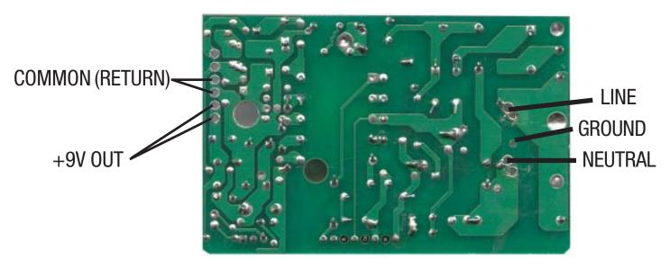
**NOTE:** There is no "Ground" connection to this board The Hole in Board is for an IEC connector & Does not connect to anything
