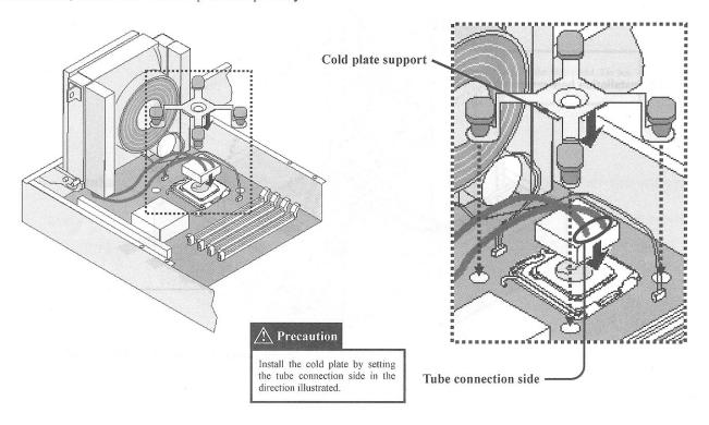
8. Insert the fastener cap until it clicks, and securely fasten the cold plate to the CPU.
