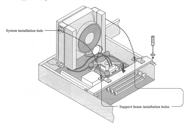
10. Put the device in the case. Adjust the installation holes of the device and the support beam, and fasten at two locations.
