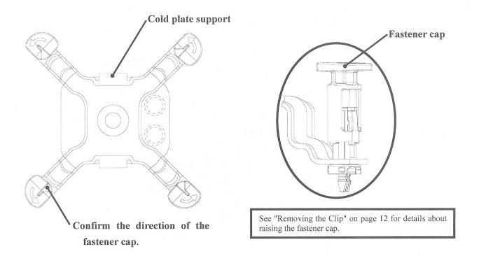
7. Adjust the cold plate so that it is in the center of the CPU. Adjust the clip so that it sits on the four open holes on the motherboard, and fasten the cold plate temporarily.
