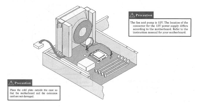
5. Apply the thermal grease to the CPU. Apply an appropriate amount of grease uniformly all over the CPU.
