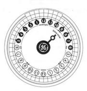
Shows timer set to turn device ON at 10 PM and OFF at 2 AM. Notice ALL segments between 10 PM and 2 AM have been pushed out. Current time is 9:00 PM.
