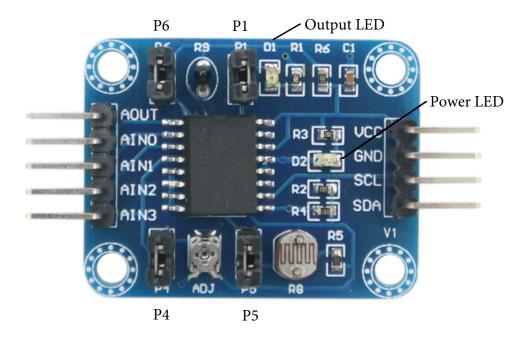
Aout: DAC Analog Output Ain0-3: ADC Analog Inputs VCC: Power supply Positive (+) 2.5~6VDC GND: Power supply Negative (-) SCL: Serial clock connection to Microcontroller SDA: Serial data connection to Microcontroller
