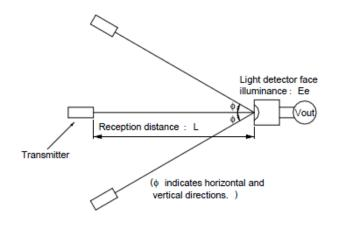
Fig. 2. Standard optical system
