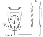
To test a diode out of a circuit, connect the Meter as follows:
