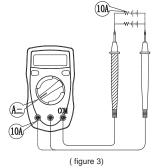
The Model UT33B: the current measurement has 3 measurement positions on the rotary switch: 200µA. 200µA and 10A.
